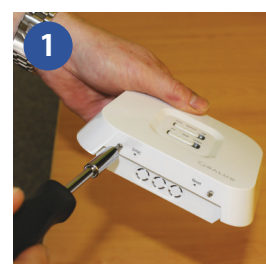
1 Loosen the screws at the bottom of the receiver unit.
